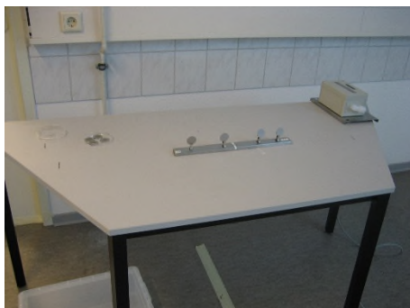
Figure 3: Position of the slats with the inoculated carrier in the test room
